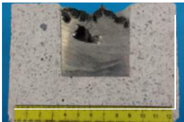
Corrosion test with fired product at 800°C, alloy 5085 (4,5%Mg)+NaCl/KCl, 8 hour test at 800°C.
