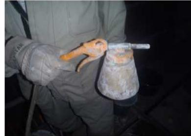
Fig 14: Spray-gun equipped with a bottle container for refractory paint application
