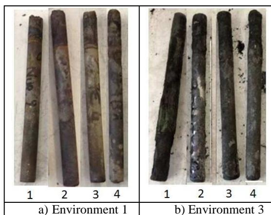
Fig 9: Metallic rods after corrosion test
