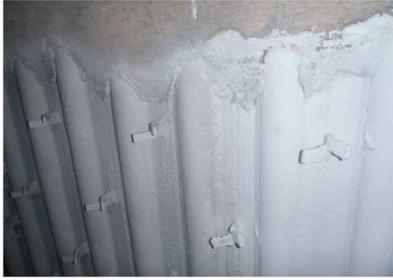
Fig 12: Coated tubes with hydraulic bond paint (right side) and benchmark product (left side).
