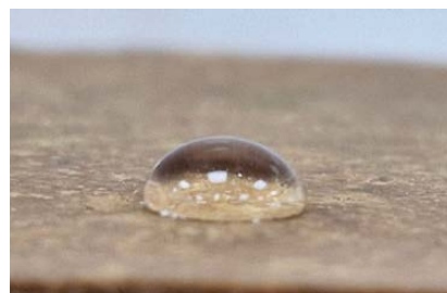
HR Series: > 90^\circ contact angle - water repelled
