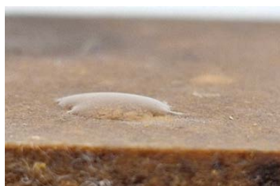
Standard brick: < 90^\circ contact angle - water absorbed
