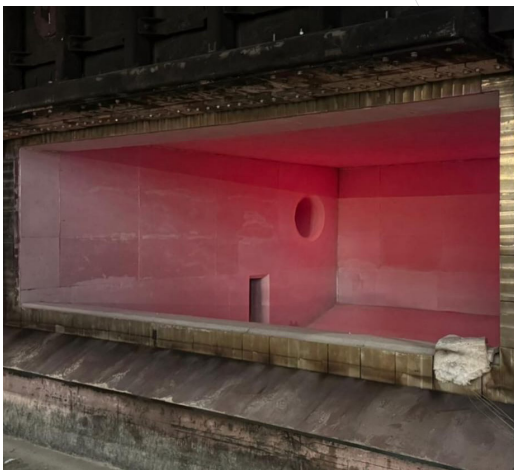
The 25-ton Aluminum melting furnace after the relining.
