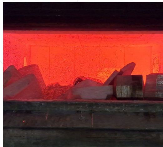
The 25-ton Aluminum melting furnace after the relining.
