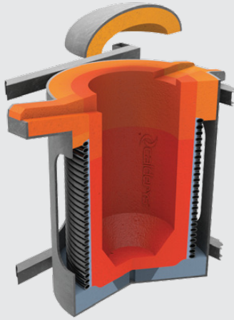
Coreless induction furnace
