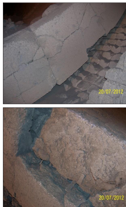
Fig 1: Tip Casting Monolithic after use
