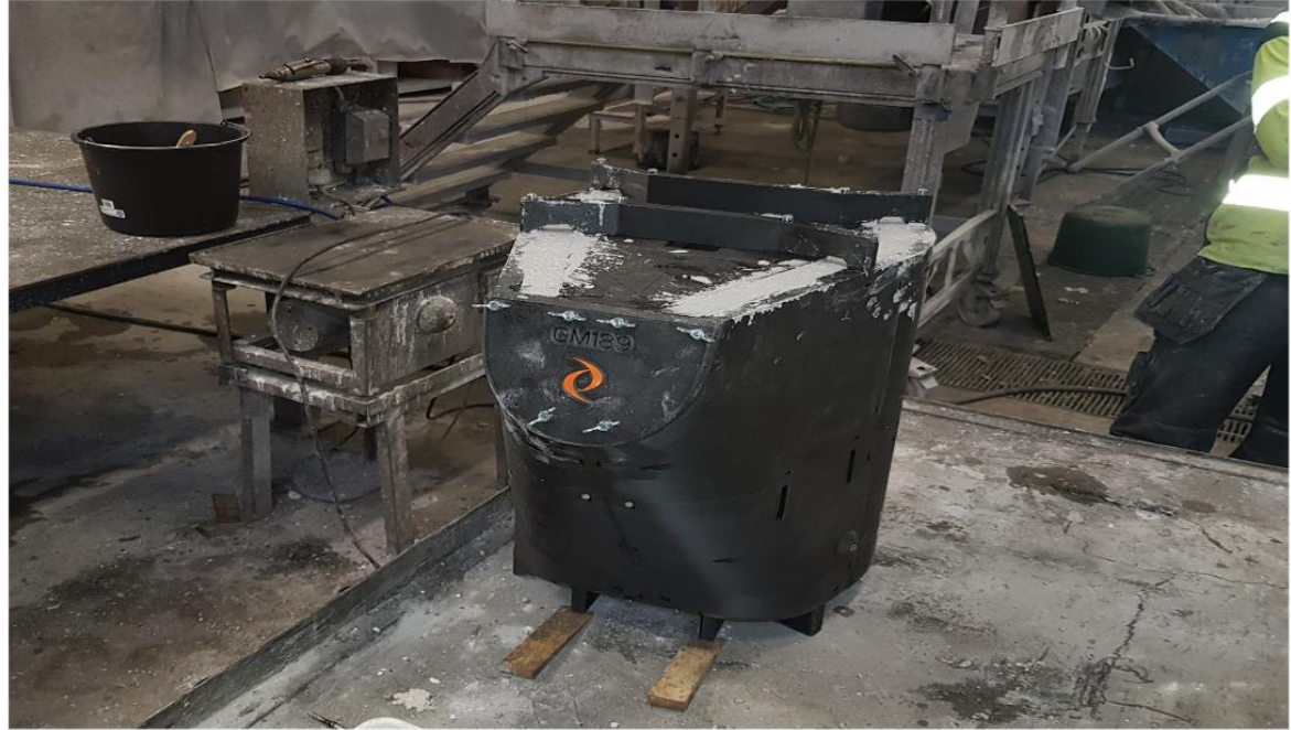
3D printed molds ready for casting
