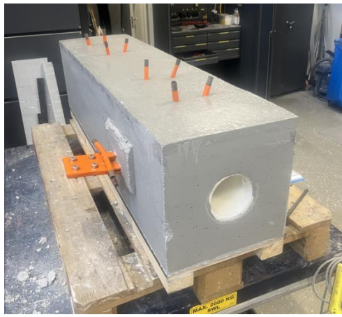
Full mechanic and refractory repair of induction heaters
